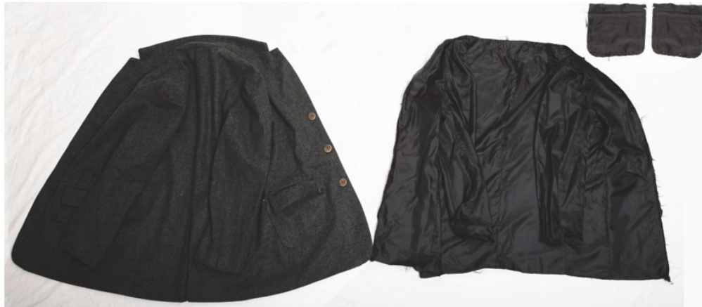
left — biological nutrients (wool fabrics, organic cotton threads, Tagua buttons) right — technical nutrients (polyester fabrics, polyester threads)
