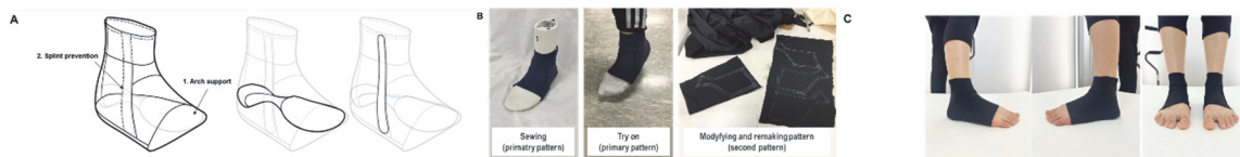
Figure 2. Production process: (a) ideation and concept; (b) base layer creation; and (c) sleeve integration
