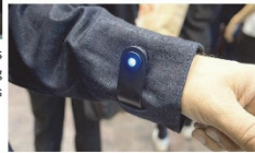
Google and Levi's commuter trucker jacket , uses conductive yarn to build touch and gesture sensitive areas on the sleeve to control connected devices like a phone.
